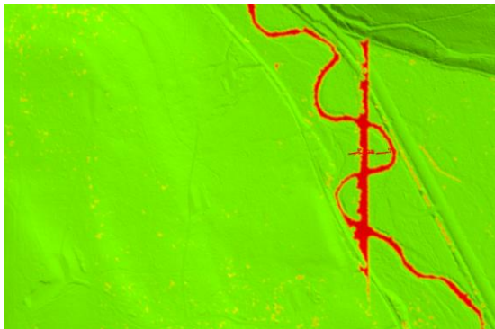
Bare-earth (class 2 + class 8 + class15) model with density information (red = sparse data)
