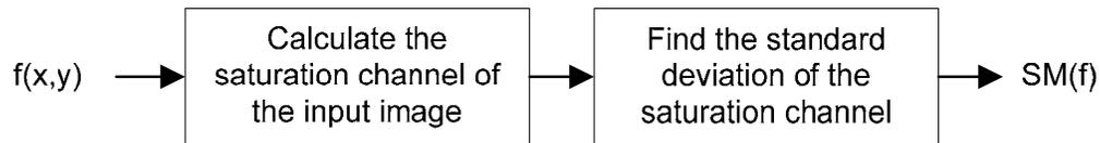
Figure 4.3.1 – Saturation metric
