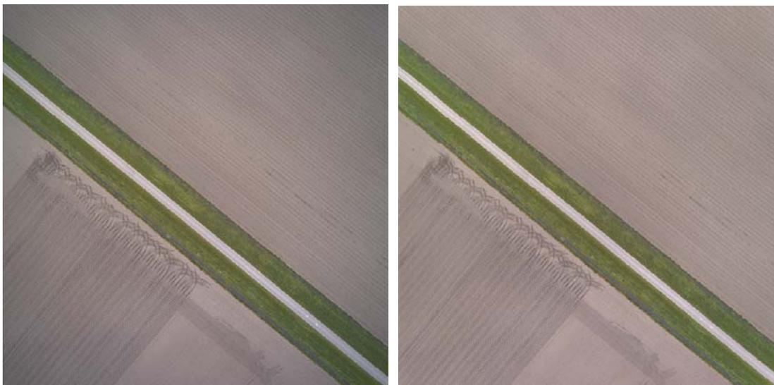
**Figure 5.2.21.2.** Raw Image (L) and Lens Falloff Corrected (R)
