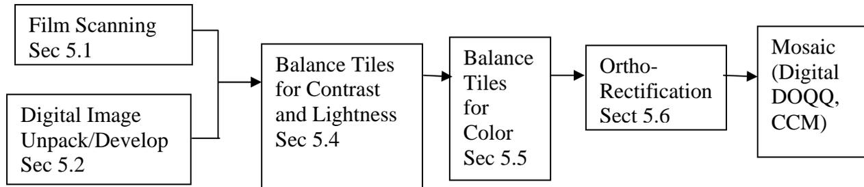
**Figure 5.1** Suggested Image Processing flow
