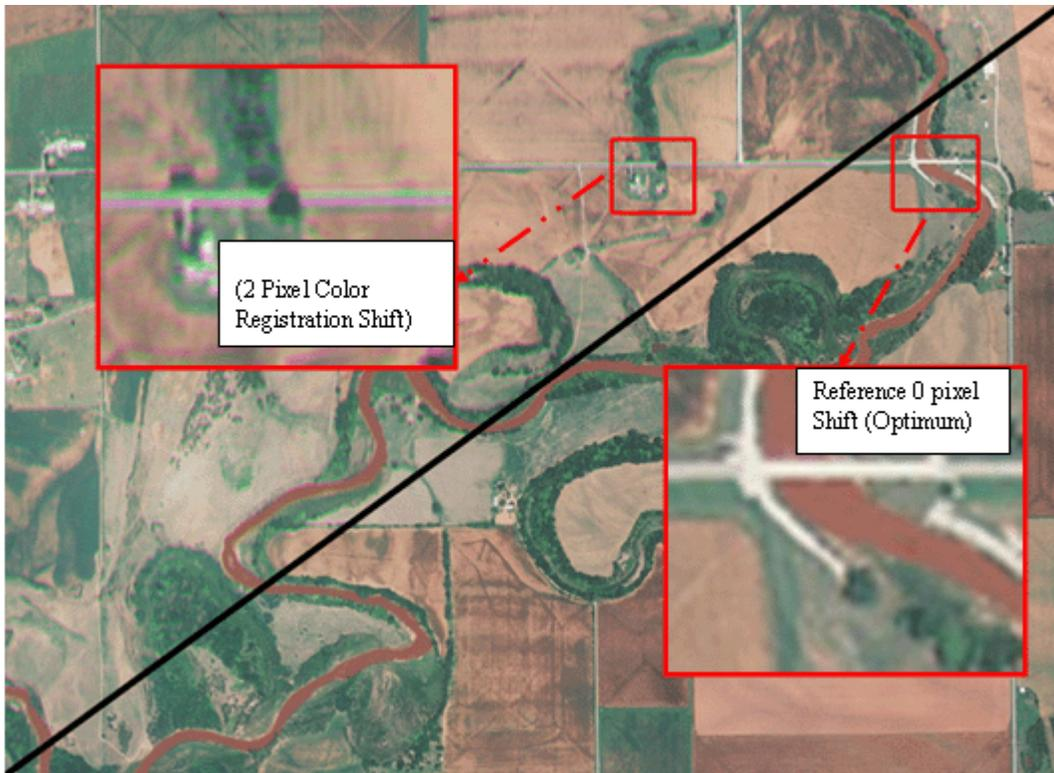
**Figure 5.2.1.1.** Illustration of Color registration shift versus an Optimum image
