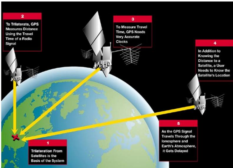
*The accuracy of the Global Positioning System depends on data NGA provides to the Department of Defense on the orbit of each satellite in the constellation.*
