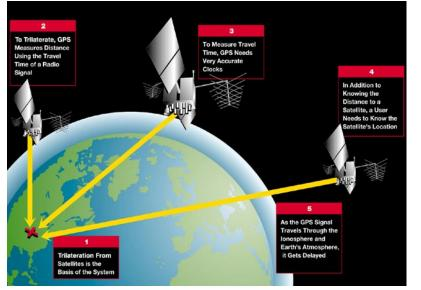
The accuracy of the **Global Positioning** System depends on data NGA provides to the Department of Defense on in the constellation.
