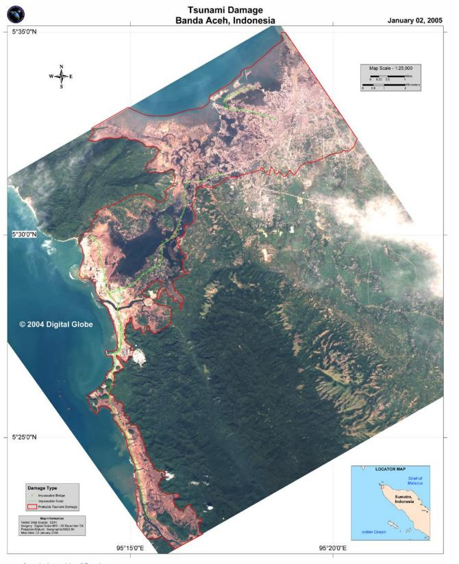
A coded graphic of Banda Aceh provided to relief workers shows the damage area outlined in red, impassable roads marked in green and yellow circles over washed out bridges.
