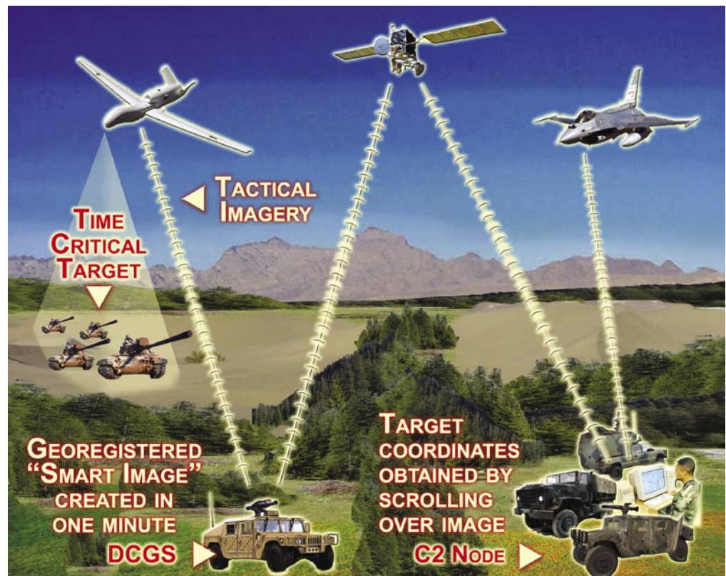
A typical concept of operations for Gridlock shows an unmanned aerial vehicle (upper left) gathering imagery of a time-critical target. Using Gridlock, warfighters in the Distributed Common Ground System (DCGS) create a georegistered smart image in one minute. They distribute the targeting information to an appropriate command-and-control targeting authority (C2 Node), which transmits the precise coordinates to the fighter pilot (upper right).
